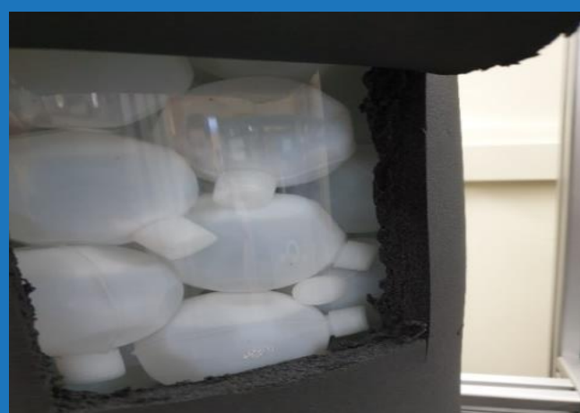
Freezing of synthesized paraffin-based PCM in lab-scale EPCM LTES test rig
