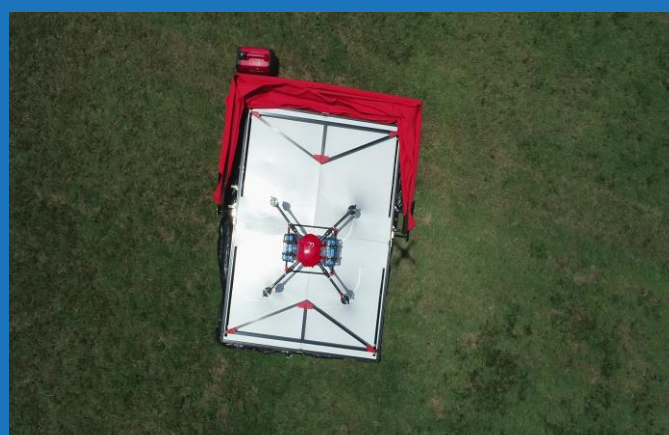
Figure 4. A docking station with coverage system and auto charging mechanism.
