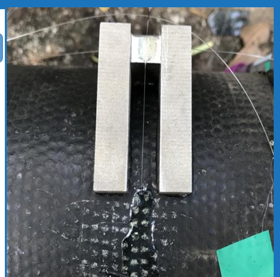
Figure 5: Developed fiber optic acoustic sensor being tested on-site at PowerGas' gas pipeline.
