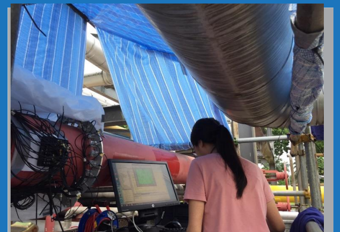
On-site trial of the developed solution using guided wave tomography at Jurong Island
