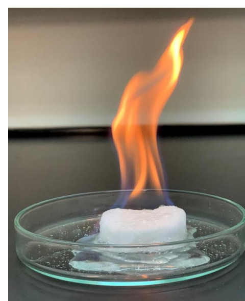
A burning Solidified Natural Gas (SNG) Pellet
