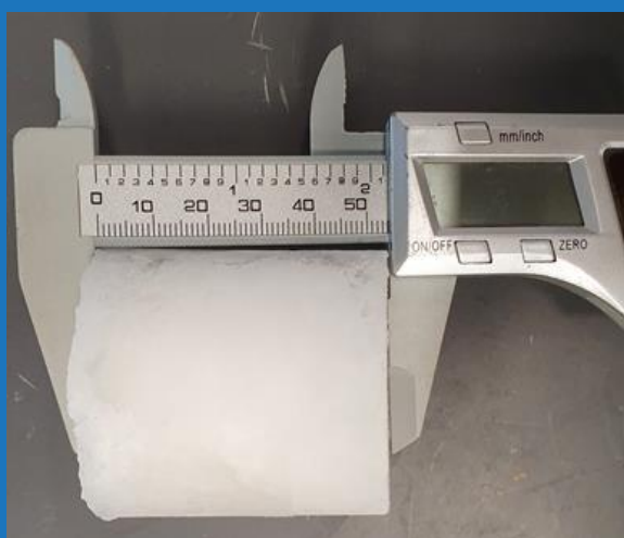
A cylindrical SNG pellet produced using a bench-scale SNG technology prototype
