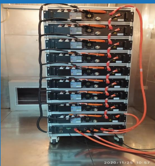
Figure 3: Chamber testing of ESS
